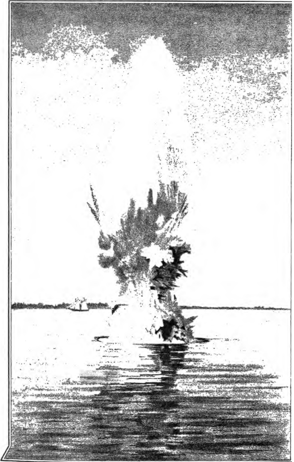
Charge, 276 lbs. Mortar Powder. Mine resting on bottom in water 10 feet deep. Height of Jet about 280 feet.
